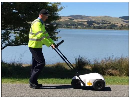
WDM's TM2 surface texture measurement device is the result of extensive research and development linking surface texture traditionally measured using the sand patch test with high-speed laser texture measurement commonly used in pavement condition assessment.
